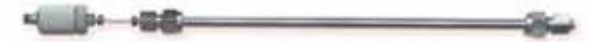
NewGuard cartridges directly coupled to a 220 mm MPLC cartridge and connected externally to a 250 mm conventional column.
