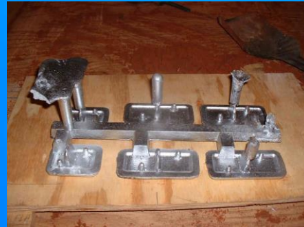
Figure 16.129 Components of a running and feeding system
