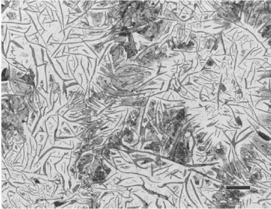
FIGURE 3.10 Examples of ferritic gray iron specimens, both are etched with 2% nital. The specimen at left has 30% pearlite while the specimen at right is fully ferritic. The magnification bar lengths are 100 and 20 \mu\text{m} , left and right.
