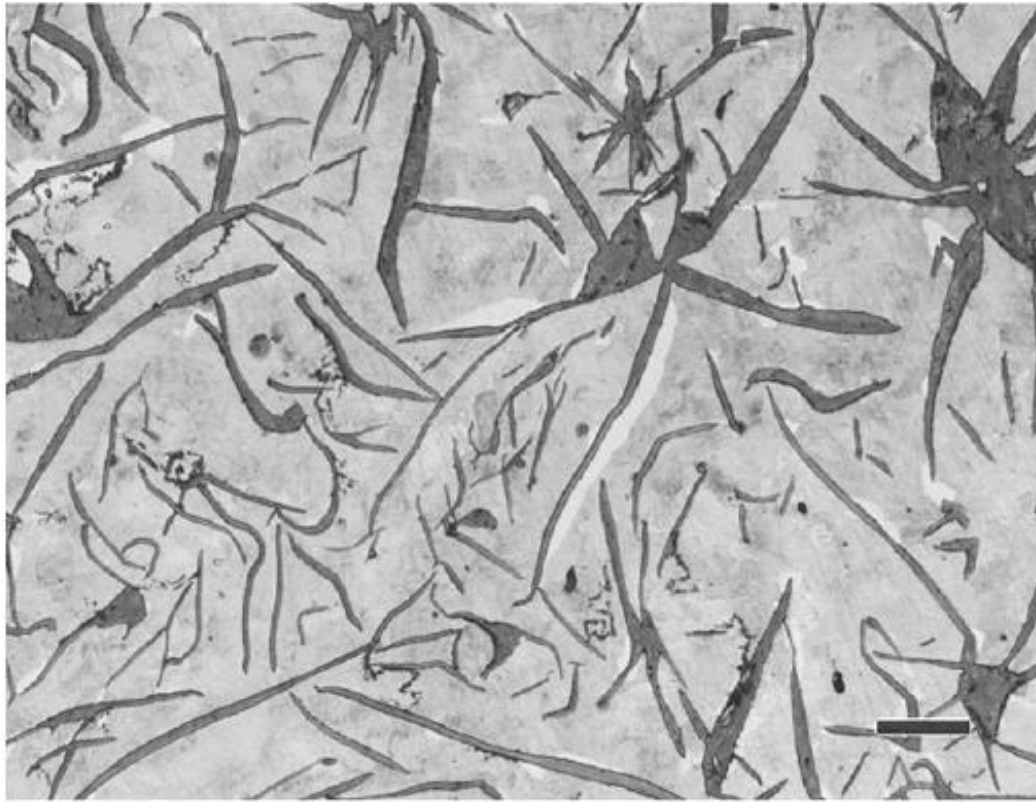
FIGURE 3.9 Examples of pearlitic gray irons with small amounts of ferrite (1.5% at left and 18% at right). Both specimens were etched with 2% nital. The magnification bar lengths are 50 and 20 \mu\text{m} , left and right.
