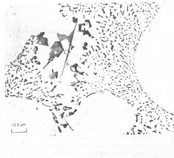
Fig. 3-38. Absence of lamellar structure in Al-Si alloy. #4 on scale.
