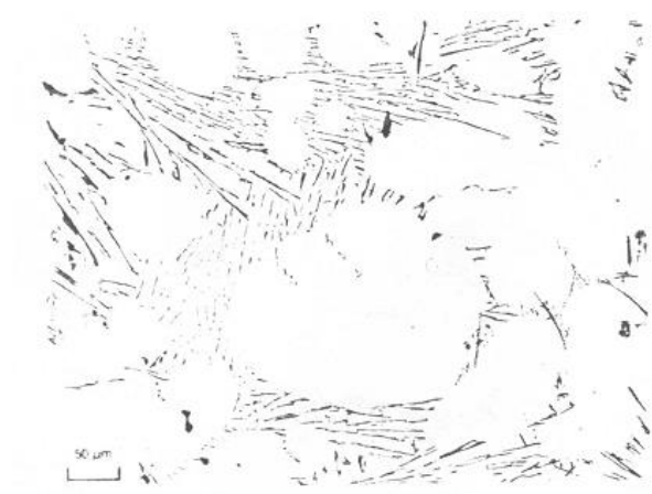
Fig. 3-36. Lamellar structure of Al-Si alloy, #2 on scale.
