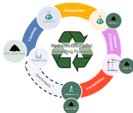
Fig.1. Schematic representation of the hydrometallurgical process for the treatment of waste lithium-ion batteries.
