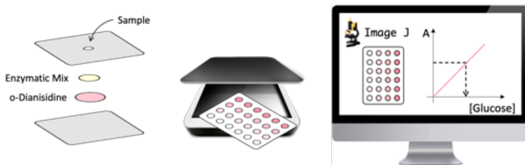
Fig. 1. Schematic representation of the assembly and determination procedure for the quantification of glucose with the developed device.
