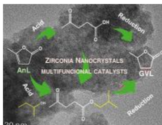
Fig.1. Integrated catalytic conversion of biomass derived \alpha -angelica lactone (AnL).
