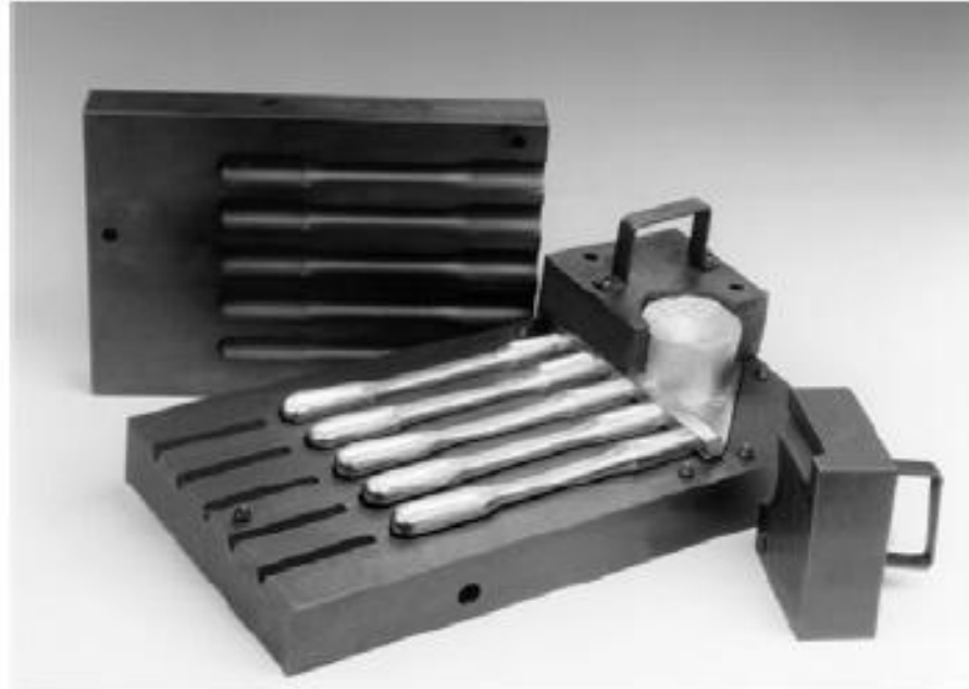
Figure 6: A multiple test bar mold is used to cast specimens for mechanical testing. (N-Tec)
