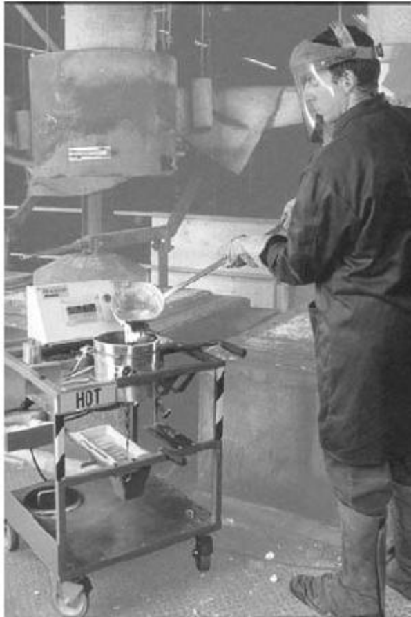
Figure 3: The Qualiflash test measures molten metal fluidity semi-quantitatively.
