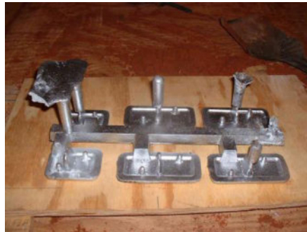
Figure 16.129 Components of a running and feeding system
