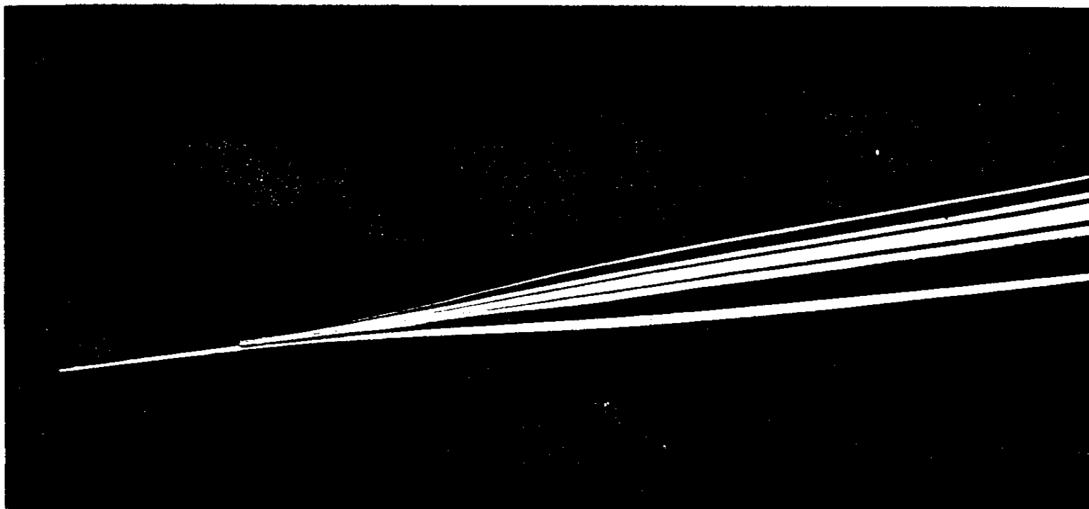
Figure 77. (a) A potassium ion-selective microelectrode of the double-barrel type. (According to J. L. Walker). (b) A micrograph of the capillary tip of a double-barrel ammonium-selective microelectrode (by permission of D. de Beer)
