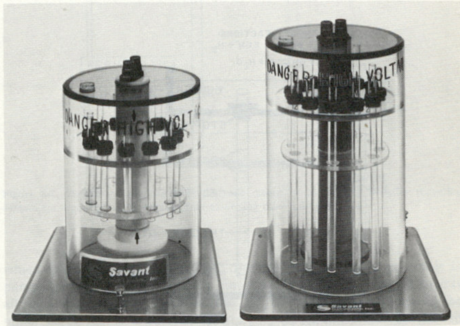
Figure 6-6. Commercially available chambers for acylamide gel electrophoresis of short and long gels. Arrows in the left apparatus point to the platinum electrode wires. (Courtesy of Savant Instruments, Inc., Hicksville, N.Y.)
