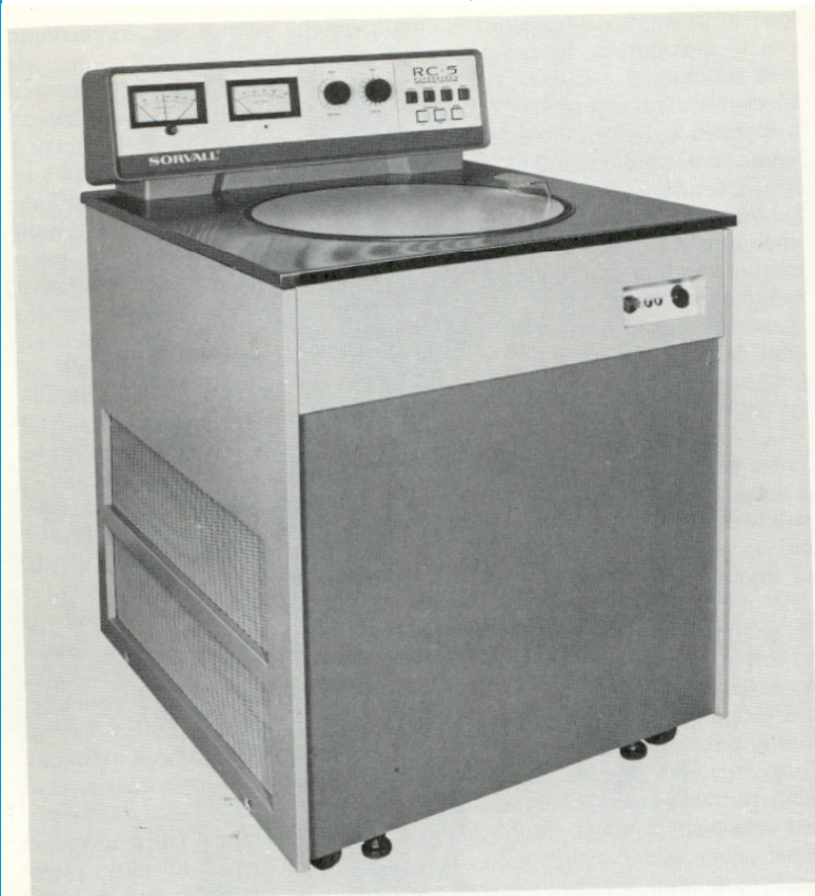
Figure 9-3. Sorvall refrigerated highspeed centrifuge. Meters display the temperature and running speed; the two dials are used for selecting the speed of centrifugation. (Courtesy of DuPont Instruments, Newtown, Conn.)
