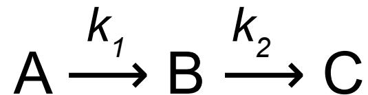
$$\frac{d[A]}{dt} = -k_1[A] \quad \frac{d[B]}{dt} = k_1[A] - k_2[B] \quad \frac{d[C]}{dt} = k_2[B]$$
