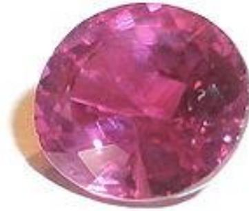
Rubí: ( $\text{Al}_2\text{O}_3:\text{Cr}$ )
