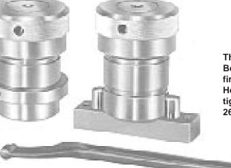
The 4744 and 4749 Bombs can be held firmly in an A285AC Holding Fixture while tightening the cap with a 264AC2 Hook Spanner
