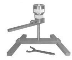
The A263AC Spanner-Jack holds the 4746 Bomb firmly during opening and closing operations and provides a convenient tool for pressing the PTFE cup out of the body.
