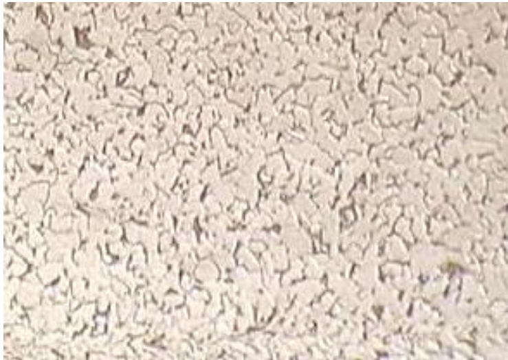
Fig. 52. — Steel. Carbon 0.10 per cent. Magnified 100 diameters. (E. L. Reed.)
