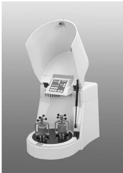
Figure 5.10 Benchtop pulverizing mill used for mechanical alloying. (Courtesy of Fritsch GmbH, Idar-Oberstein, Germany.)
