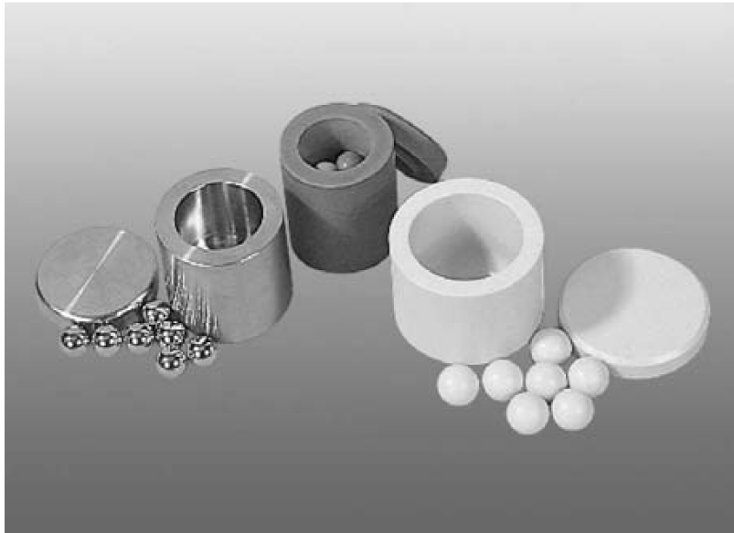
Figure 5.11 Balls and containers of different materials used for benchtop pulverizing mill. (Courtesy of Fritsch GmbH, Idar-Oberstein, Germany.)
