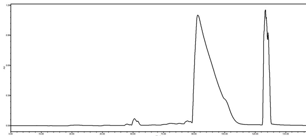
**Fig. 6.** Chromatogram from RP-HPLC. The insulin was purified under isocratic conditions - mobile phase A: 2000 ml of 0.2 M sodium sulphate solution pH 2.3 preheated in warm water to 25 °C - 30 °C with 440 ml of acetonitrile, pH 2.3. Mobile phase B: 1250 ml of 0.2 M sodium sulphate solution pH 2.3 preheated in warm water to 25 °C - 30 °C with 1250 ml acetonitrile, pH 2.3. Detector wavelength: 214 nm. The insulin peak is from about 90 to 105 min (x-axis).
