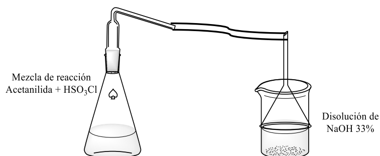
Figure 2. Gas trap (HCl) for the synthesis of N-acetyl sulfanylium chloride.
