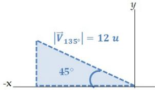
$$\cos 45^\circ = \frac{|\vec{v}_x|}{|\vec{v}_{135^\circ}|} \therefore |\vec{v}_x| = 12u * \cos 45^\circ = 8.49 u \quad \text{sen } 45^\circ = \frac{|\vec{v}_y|}{|\vec{v}_{135^\circ}|} \therefore |\vec{v}_y| = 12u * \text{sen } 45^\circ = 8.49 u$$
