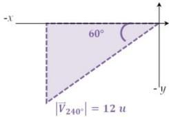
$$\cos 60^\circ = \frac{|\vec{v}_x|}{|\vec{v}_{240^\circ}|} \therefore |\vec{v}_x| = 12u * \cos 60^\circ = 6.00 u \quad \text{sen } 60^\circ = \frac{|\vec{v}_y|}{|\vec{v}_{240^\circ}|} \therefore |\vec{v}_y| = 12u * \text{sen } 60^\circ = 10.39 u$$
