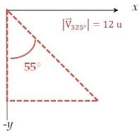
$$\text{sen } 55^\circ = \frac{|\vec{v}_x|}{|\vec{v}_{325^\circ}|} \therefore 12u * \text{sen } 55^\circ = 9.83 u$$
