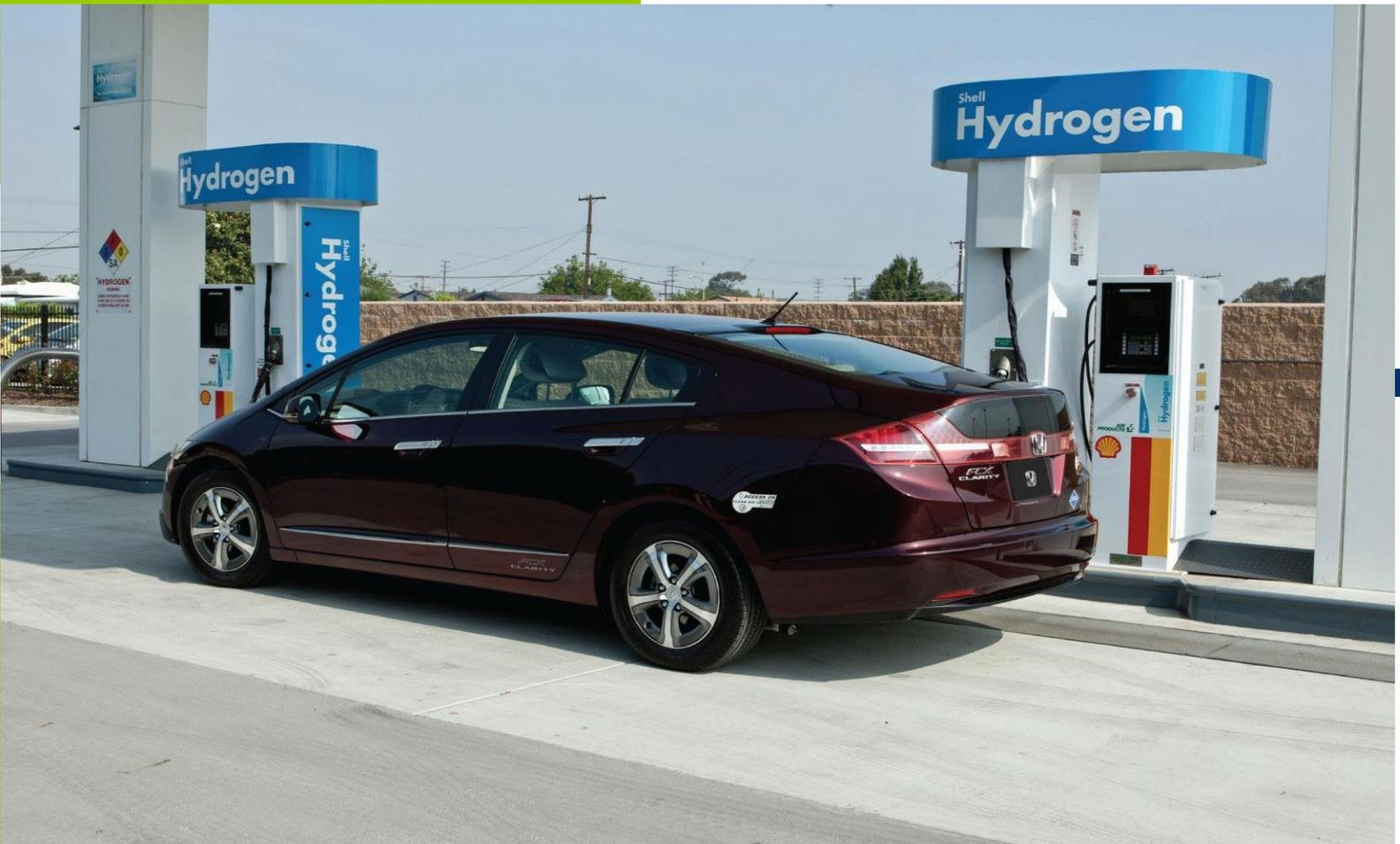
The Honda FCX Clarity, a fuel-cell- powered automobile available to the public, albeit in limited quantities. A fuel cell converts hydrogen fuel into electricity to drive the motor attached to the wheels of the car.
