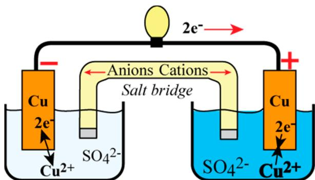
**Figure 7.** Schematic of a copper-based concentration cell. The equilibration of the  $\text{Cu}^{2+}$  concentrations is spontaneous, and the associated reduction in the total Gibbs free energy drives the cell processes. The electrical work is supplied as heat from the surroundings.
