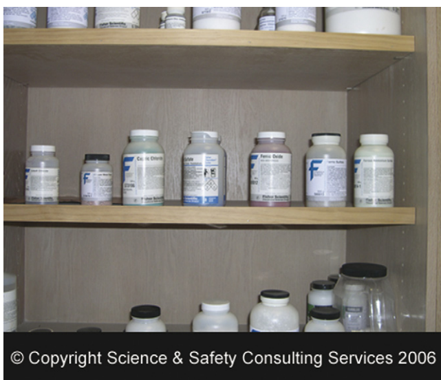
Figure 3. Correct chemical storage system: bottles labeled, appropriate chemicals for secondary school laboratories, compatible chemical storage. Courtesy S&SCS, used with permission.
