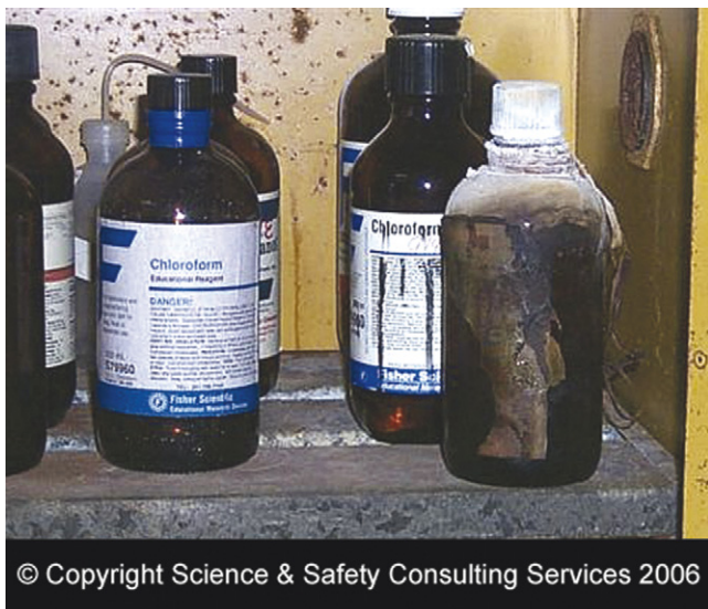
Figure 2. Incorrect chemical storage system: unlabeled bottles, inappropriate chemicals for secondary school laboratories and incompatible chemical storage, courtesy Larry Cockrell, NCDPI, used with permission.
