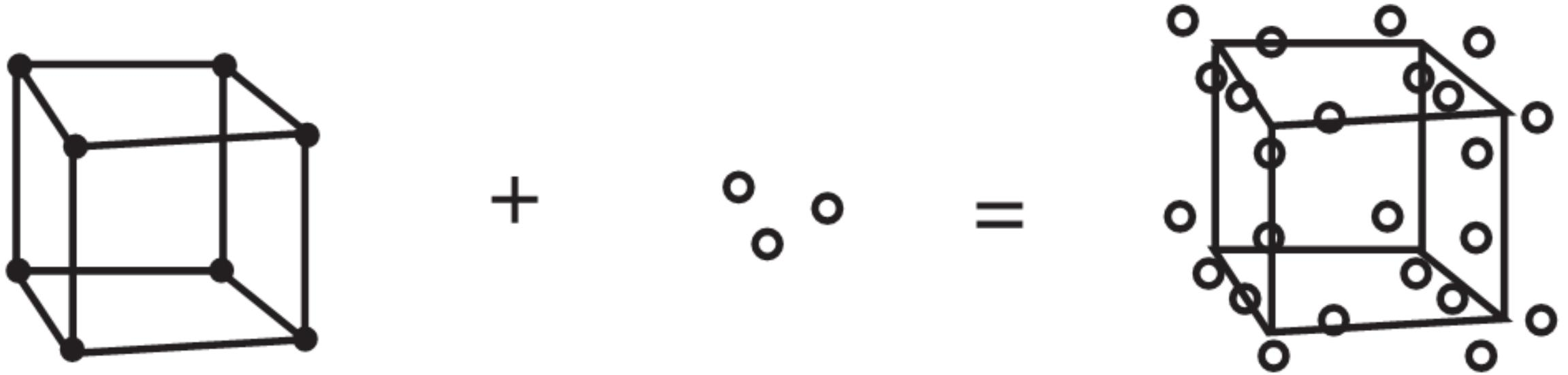
Figure 2.6 Lattice plus basis yields a crystal structure.
