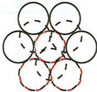
ABABABAB Two-layer repeat Hexagonal close-packed
