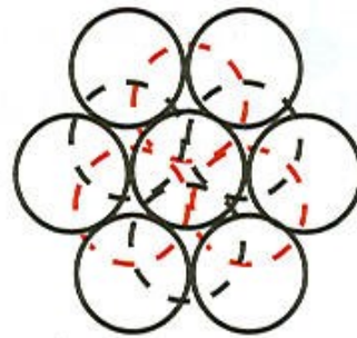
ABCABCABC Three-layer repeat Cubic close-packed
