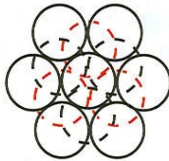
ABCABCABC Three-layer repeat Cubic close-packed
